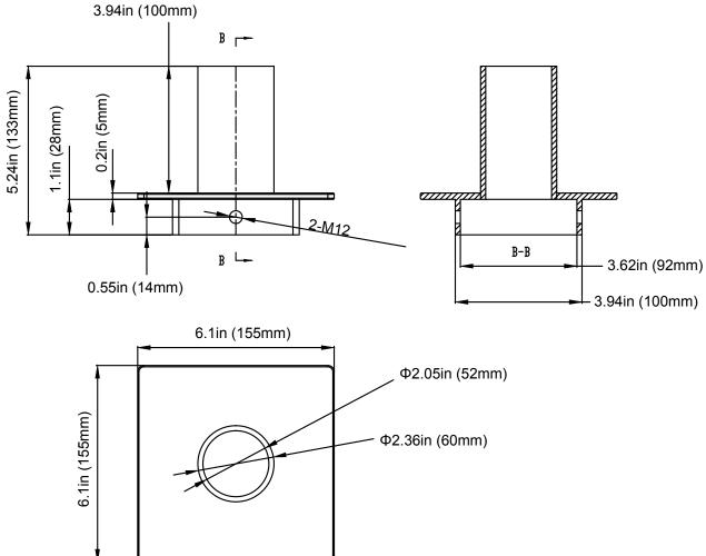
Mount - 4" Square Tenon Vertical to 2-3/8"(2.5) triple heads at 180deg
