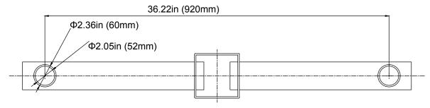
Mount - 4" Square Tenon Vertical to 2-3/8"(2.5) triple heads at 180deg
